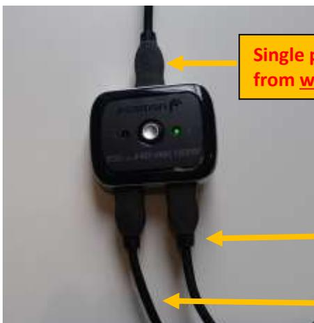
Single port: for attaching a HDMI cable from wall socket to the HDMI switch
