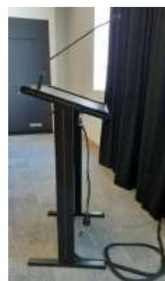
Plug the laptop power cord into the laptop, and cord which hangs down from the lectern. Plug the HDMI cord hanging from the lectern into the right-hand side of the laptop.
